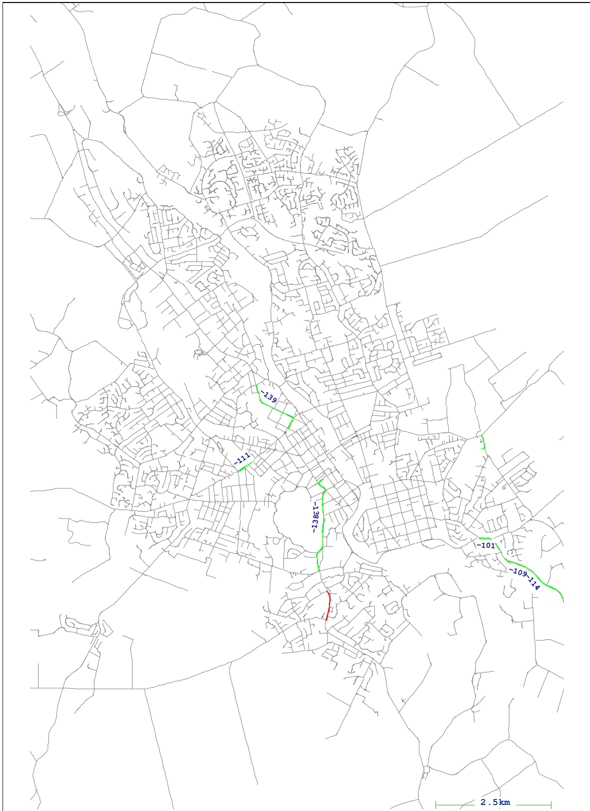
Waikato Regional Transportation Model Three Step vs Four Step Hourly Volume Changes Hamilton - Morning Peak Figure 9 Gabites Porter Traffic Design Group
